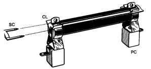
These flexible clips, of special alloy, provide effective protection against corrosion and extreme working temperature.
