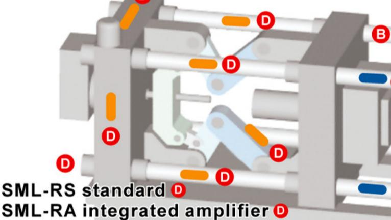
Measuring Strain Ring for strain measurement
