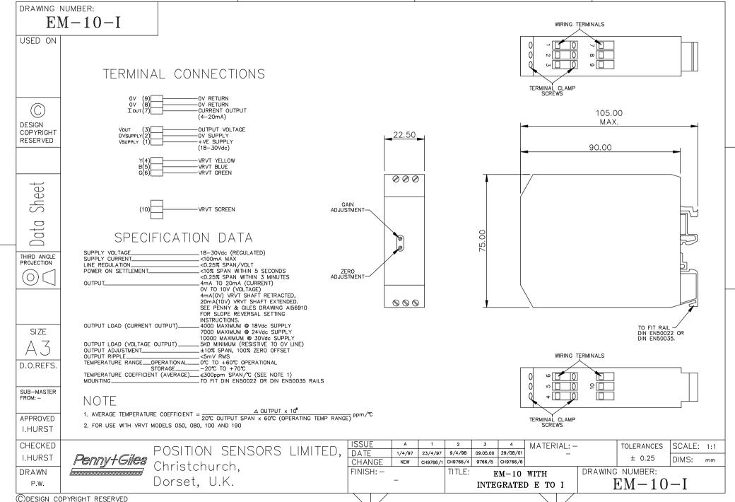
.OV TO 10V (VOLTAGE) FOR FULL VRVT ELECTRICAL SHAFT DISPLACEMENT (OV RETRACT, 10V EXTEND). SEE PENNY & GILES DRAWING A156247 FOR OV TO 5V, ±5V AND SLOPE REVERSAL OUTPUT SETTING INSTRUCTIONS. OUTPUT LOAD (VOLTAGE OUTPUT). 5KΩ MINIMUM (RESISTIVE TO OV LINE) OUTPUT ADJUSTMENT ±10% SPAN, 100% ZERO OFFSET OUTPUT RIPPLE <5mV RMS
